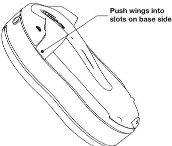
To remove the clip press one of the wings away from the body.
