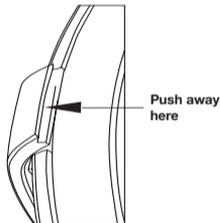
To fit the neck cord remove belt clip and thread the cord as shown, and replace the belt clip. The neck cord has a safety release Feature to avoid you getting trapped by the cord.
